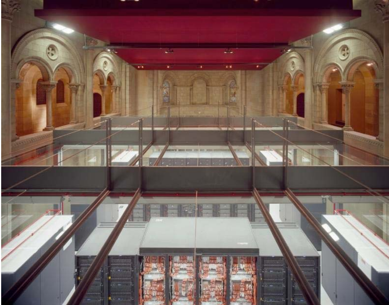
MareNostrum Cluster in Barcelona. The central switch has 2560 host ports. Photo courtesy of IBM.
